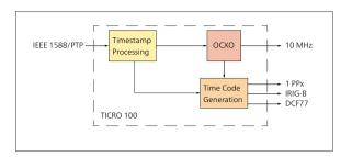
Simply assign the time code or time reference signal required by your device to an optical, coaxial or optocoupler output using TICRO 100's web interface.
