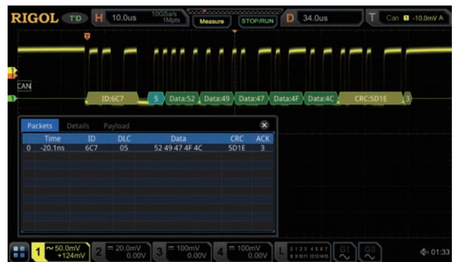
The CAN trigger helps you capture the CAN bus signal in the waveform
