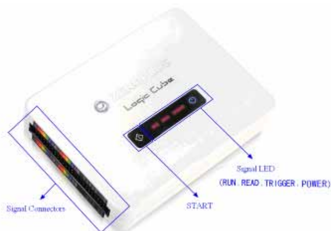
Fig. 1-12: A View of the ZeroPlus Logic Analyzer LAP-C Series. See Fig 1-11 for detailed information on the Signal Connectors
