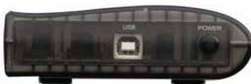
Fig. 1-10 Side view of Zeroplus Logic Analyzer, which draws its power from the USB connection.
