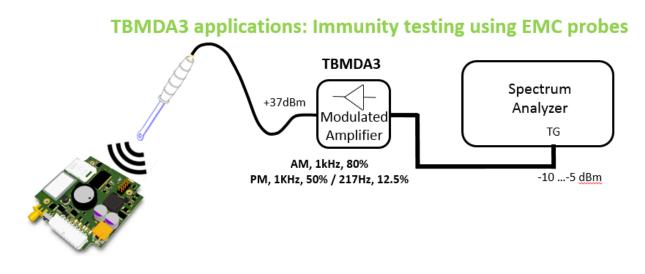
Figure 7 – immunity testing set up
