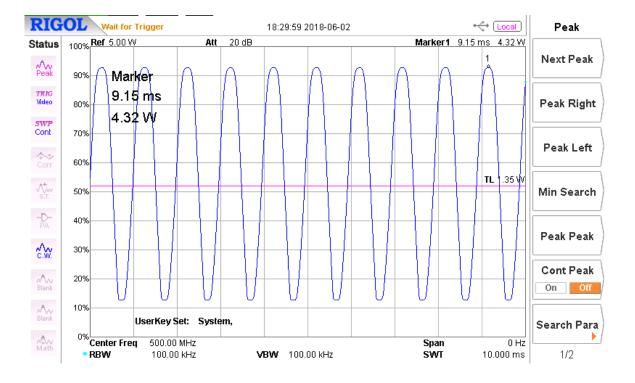
Figure 2 – 1 kHz, 80 % AM envelope, 500 MHz
