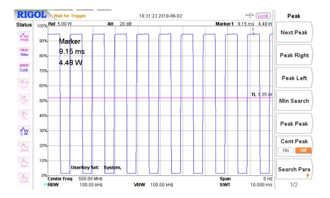
Figure 3 – 1 kHz, 50 % PM envelope, 500 MHz
