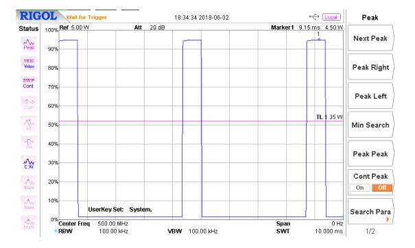
Figure 4 - 217 Hz, 12.5 % PM envelope, 500 MHz
