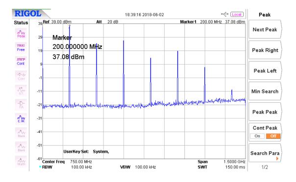
Figure 5 – CW, harmonics, 200 MHz
