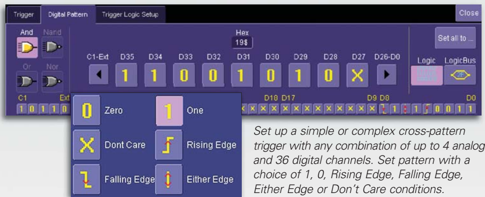
Use the oscilloscope triggers with digital channels.
